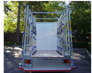
**Complete 14 ½ Foot Contractor Glazing Truck, work ready fitted to Fuso Truck**
