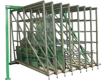
3. Use transport A-racks for transporting glass, or demountable frames for transporting window frames. These stillages allow you to load direct from your production line and store the loaded transport stillage until needed. Storage could be on a mesanine floor above your Swing rack!
